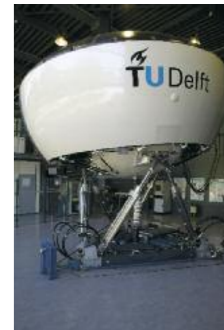
Simona Research Simulator was specially built for TU Delft and can realistically simulate all types of aircraft, helicopters and even cars.
